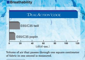
(Testing method) JIS L 1096 Breathability Test (A Method) (Fragile form method)
